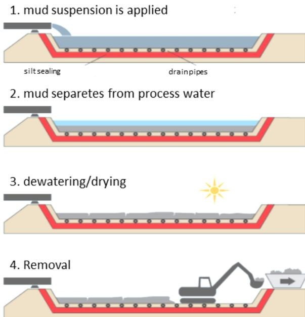
Fig. 18 Process principle of the drainage areas.
