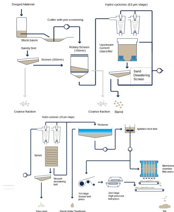
Fig. 17: How the METHA system works.
