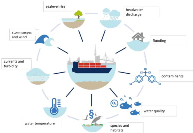
Fig. 6: Factors influencing the water depth maintenance.
