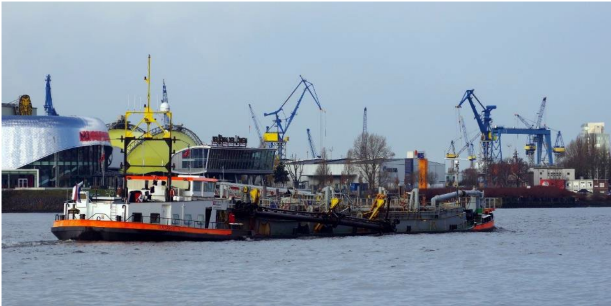
Fig. 3: The small V.d.Graaf Sr. hopper dredger is particularly suitable for narrow and confined harbour areas (Photo: Boris Hochfeld).
